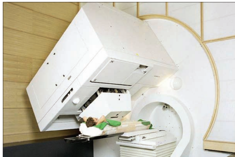
Fig. 2. The current PSI PROSCAN compact Gantry 1, which uses the active spot-scanning method. The rotating beamline gantry weighs more than 100 tonnes and is controlled to sub-millimetre precision.
